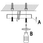
2. Drill holes, apply plastic anchors & Apply screws with a screw driver
